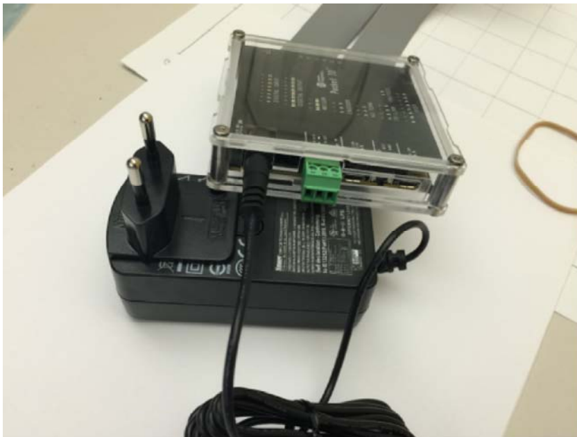
Figure 10. Pocket IO with Power Supply Connected.
